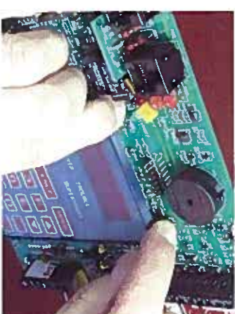
Remove bezel by pushing down on top legs to release bezel from the board.
